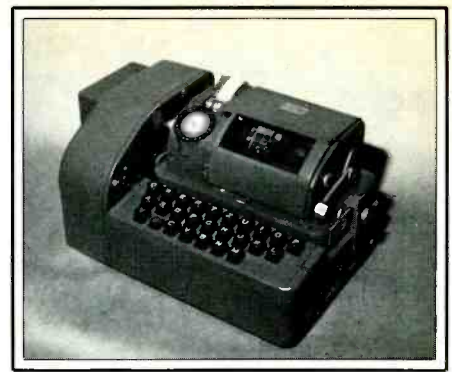
The CX-52-D shown mounted on the B-621 electric keyboard base comprised the BC-621 unit.
