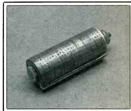
Hard to believe that this simple ciphering device was used by the U.S. Army as late as 1939. It had been invented by Thomas Jefferson.
