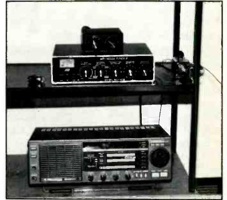
Fig. 4. Test set-up showing MW/LW and SW tuners, three-position coax switch and receiver.
